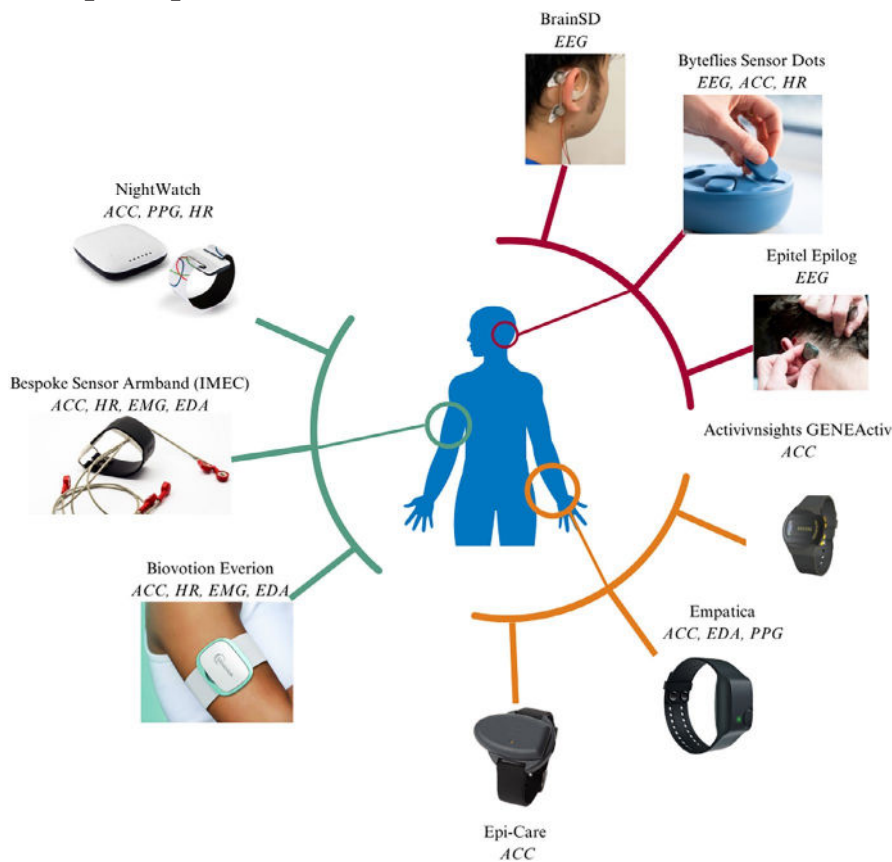
FIGURE 3 Devices appearing in the articles included in this review. Byteflies Sensor Dots may not be used only on the head; different locations are possible. Devices starting from the top and going clockwise: (1) Brain Seizure Detection (BrainSD): Lehnen J et al. 2024; (2) Byteflies Sensor Dots: byteflies.com ; (3) Epitel Epilog: Frankel MA et al. 2021; (4) Activinsights GENEActiv: activinsights.com ; (5) Empatica: empatica.com ; (6) Epi-Care: danishcare.dk ; (7) Biovotion Everion: Gashi S. et al. 2024; (8) Bespoke sensor armband (IMEC): imec-int.com ; and (9) NightWatch: nightwatchepilepsy.com . ACC, accelerometry; EDA, electrodermal activity; EEG, electroencephalography; EMG, electromyography; HR, heart rate; PPG, photoplethysmography. *Except SmartWatch by SmartMonitor, where picture was not available.
